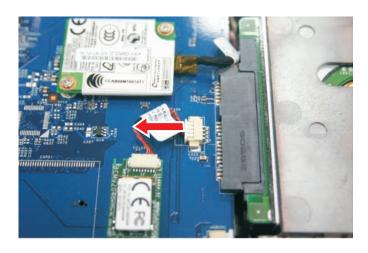
8 The Bluetooth module is glued to the system board. Carefully pry loose the Bluetooth module from the system board using a flat blade screw driver or a plastic scribe.
