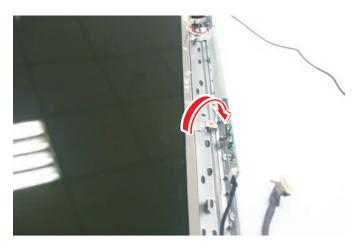
9 Disconnect the cables from the inverter board.
