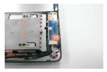
9 Release from latch and remove the USB board from the base enclosure.
