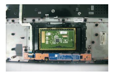
Insert a small flat-blade screwdriver or non-marring scribe between the touchpad board and the palm rest's underside, and carefully pry the board loose.
