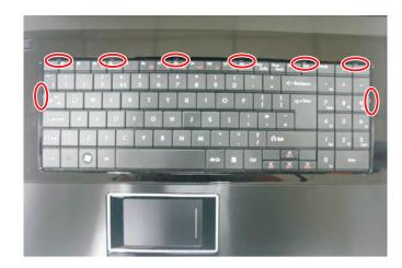
5 Carefully lift up and turn over the keyboard and place it on top of the palm rest.
