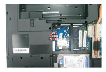
4 Use the non-marring plastic scribe to carefully push the optical drive out of the drive bay, and then slide the drive out.
