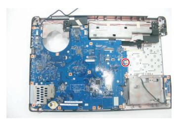
22 Carefully lift the right side of the system board and slide it out of the base panel.
