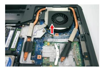
4 Loosen the spring-loaded captive screws securing thermal module. Follow the screw sequence indicated on the below images.
