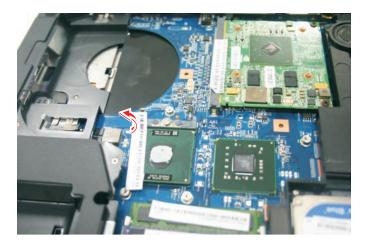
5 Use a flat-blade screw driver to turn the processor lock screw 1/4-turn counter-clockwise.
